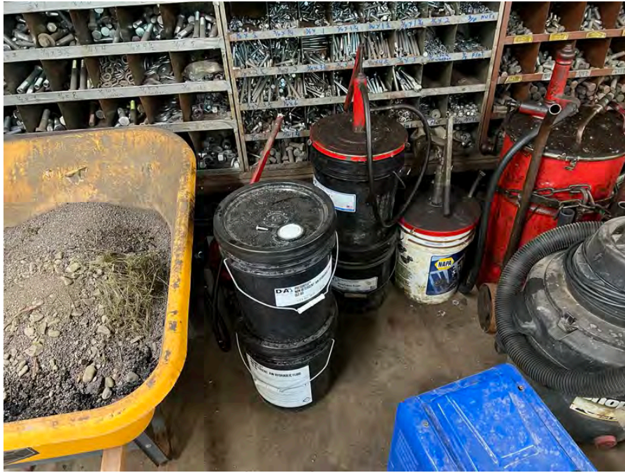
Photo 15 : 5-gallon buckets of automotive maintenance chemicals in garage of Building One
