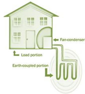
FIGURE 2-9 A geothermal air-conditioning system requires these main parts: (a) an earth-coupled portion, (b) a heat pump, (c) the building or object to be heated and cooled. (Sarah Cheney/Egg Systems)
